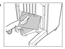
Open the exit cover of the saddle stitch unit and remove any misfed paper.
